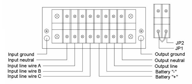
Input and output terminal block wiring diagram of three-phase 15KS/20KS
