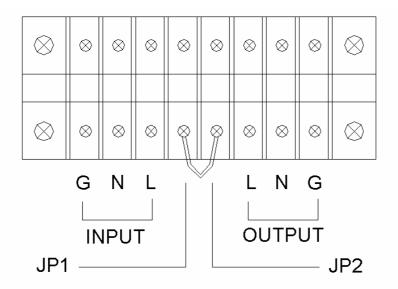
Input and output terminal block wiring diagram of H6KS(L)/H10KS(L)
