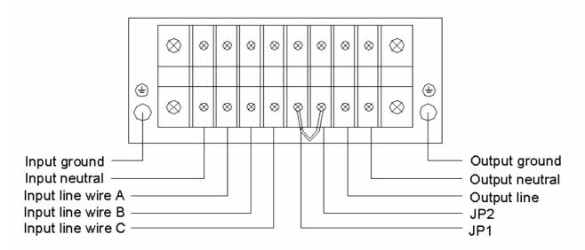
Input and output terminal block wiring diagram of three-phase 10KL
