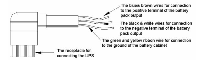
The external battery cable diagram for H6KL/H10KL (the cable may vary from different "L" models)
